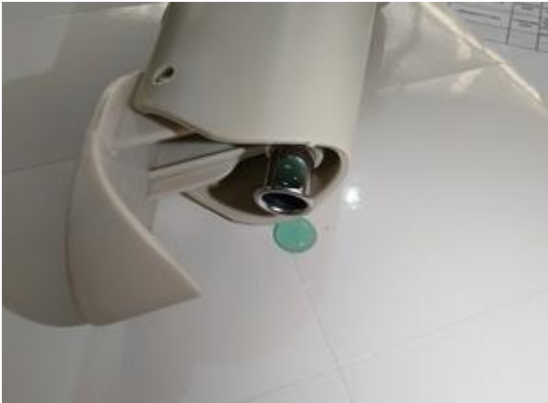
Material test-Actual finding:oil nozzle-Stainless steel 304, weight block-Stainless steel 201(1/2)
