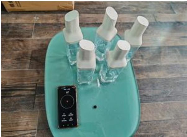
Stability test on slope-5pcs-Pass
