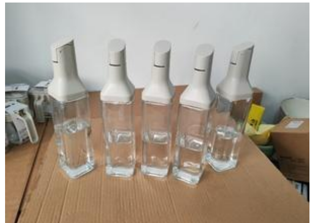
Water leakage test-5pcs-Pass
