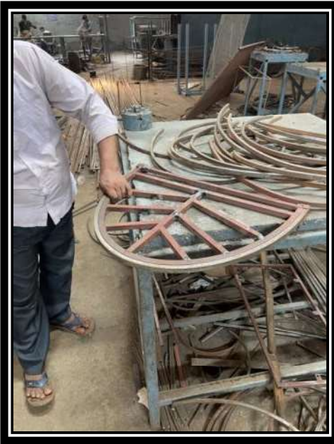
CHECKING SHAPE WITH JIG FIXTURE
