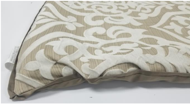
The sample demonstrates poor durability in laundering with holes noted around the Bar tacks on the back of the comforter
