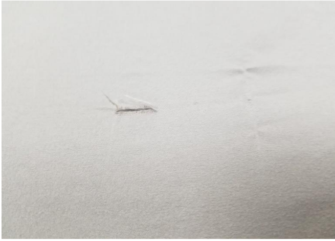
The sample demonstrates poor durability in laundering with holes noted around the Bar tacks on the back of the comforter
