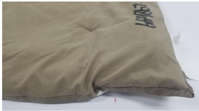
The sample demonstrates poor durability in laundering with holes noted around the Bar tacks on the back of the comforter
