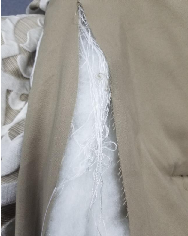
The JLA MP Odette Comforter sample submitted for testing demonstrates poor durability with the white jacquard yarns of the back side of the face fabric unraveling at the raw edge and becoming entangled in the batting
