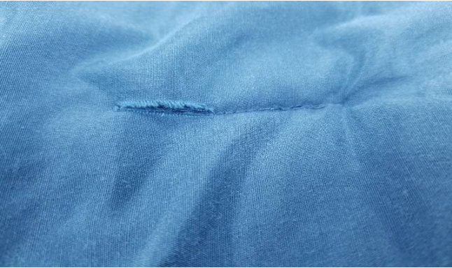
The sample demonstrates poor durability in laundering with holes noted around the Bar tacks on the back of the comforter
