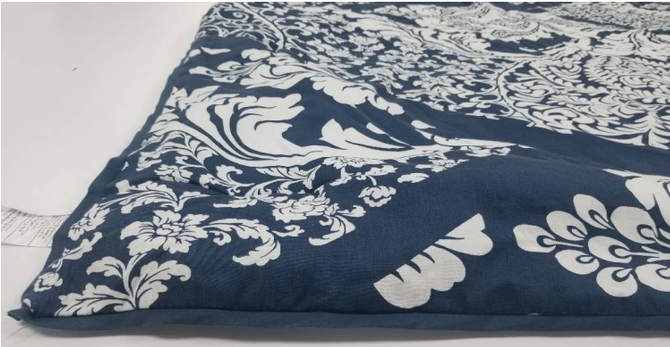
The batting used in the sample demonstrates poor durability in laundering with considerable batting migration
