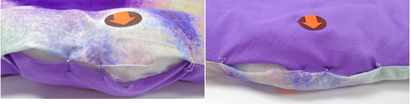
Needle damage starting runs in the fabric on several bar tacks
