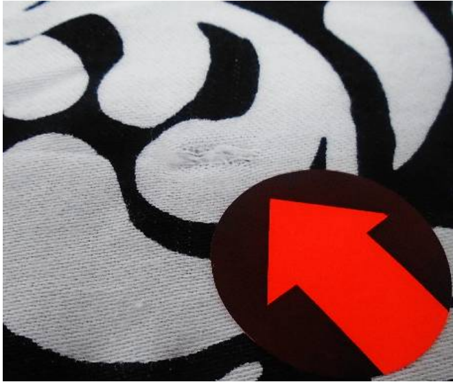
Comforter exhibits detached bar tacks with fabric damage noted
